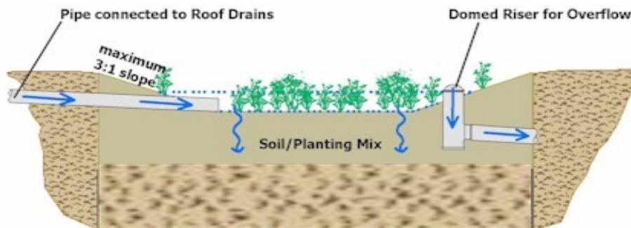
Source: Pennsylvania Stormwater BMP Manual (PADEP, 2006)
